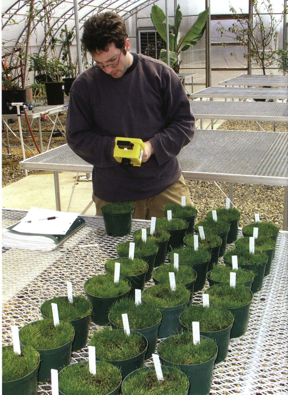
A student measures the amount of chlorophyll to determine the quality of the color in samples of grass in the greenhouse at the Turfgrass Science Complex.
