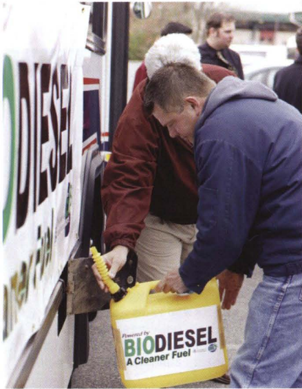
Gerry Bailey, from motor pool repairs, pours biodiesel fuel into a UConn campus shuttle bus. The bus is powered by a fuel mixture composed of 20 percent biodiesel fuel, produced using about 10 gallons of waste cooking oil used in a campus dining hall.
